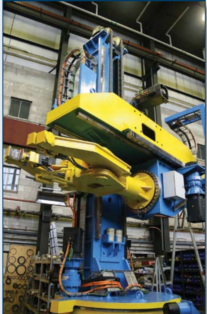
1.8 tonne capacity robot for use in aluminium smelter
